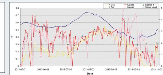
Fig. 9. Estimated fraction of flooded area ( $f_f$ ) for AMSR2 (Ka, X and C bands), SMOS (L band) and Aquarius (L band). Cosmo based  $f_f$  and Paraná River water level are shown for comparison. Zero values of  $f_f$  are set when algorithm resulted in negative values.
