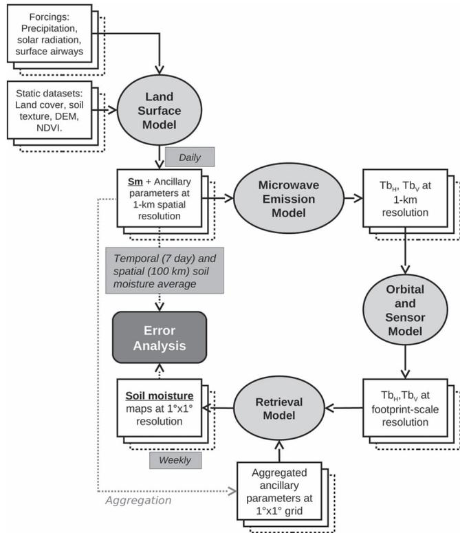
Fig. 1. OSSE block diagram.
