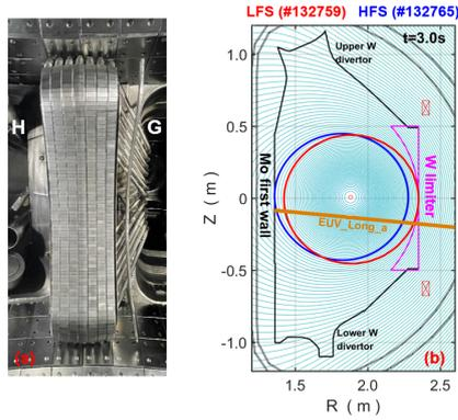
Fig. 1 (a) Front view of tungsten limiter installed between ports G and H at EAST low-field side (LFS). (b) Poloidal cross section of EAST tokamak with upper and lower tungsten divertors, tungsten limiter and molybdenum first wall. Poloidal plasma contours of Typical LFS ( $R_0 = 1.95$  m, red circle) and HFS ( $R_0 = 1.91$  m, blue circle) configurations and line of sight of fast-time-response EUV spectrometer (orange line) are also indicated.
